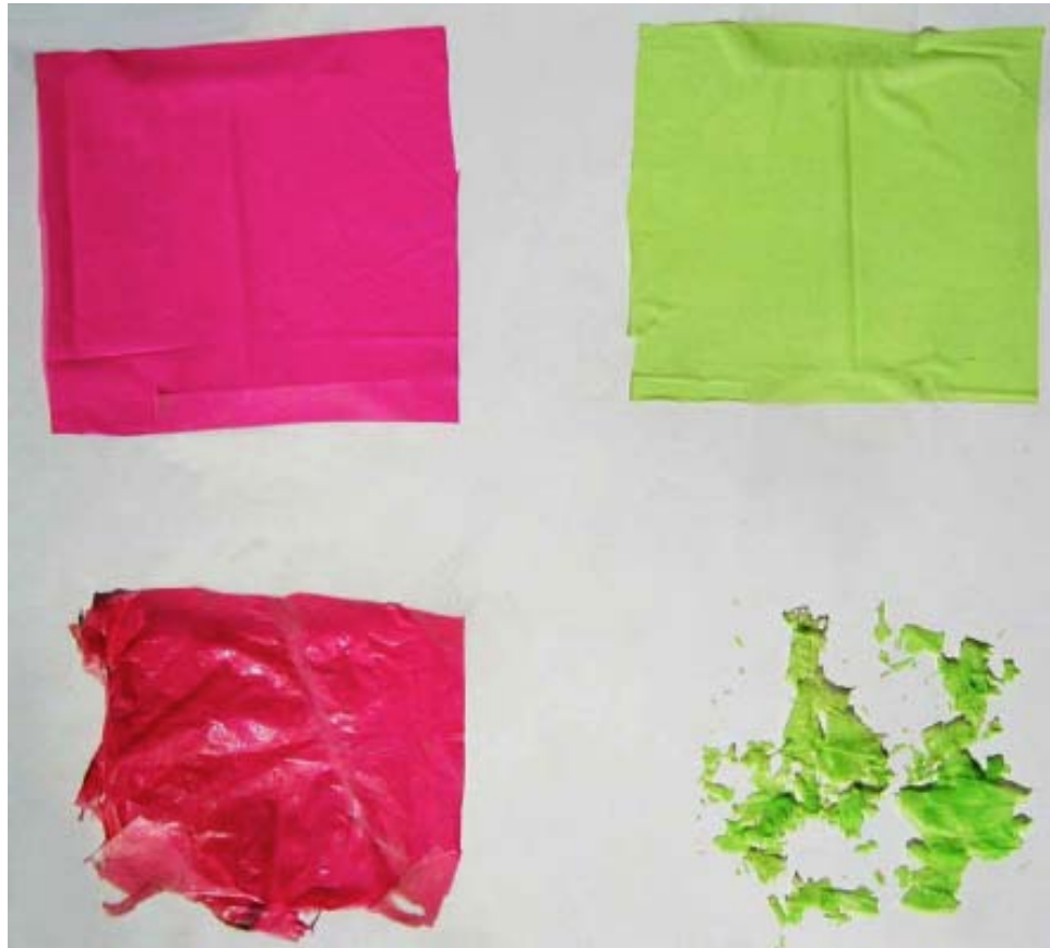
PE films with (right) and without (left) TDPA ® before (top) and after (bottom) 10 months burial in a UK landfill
